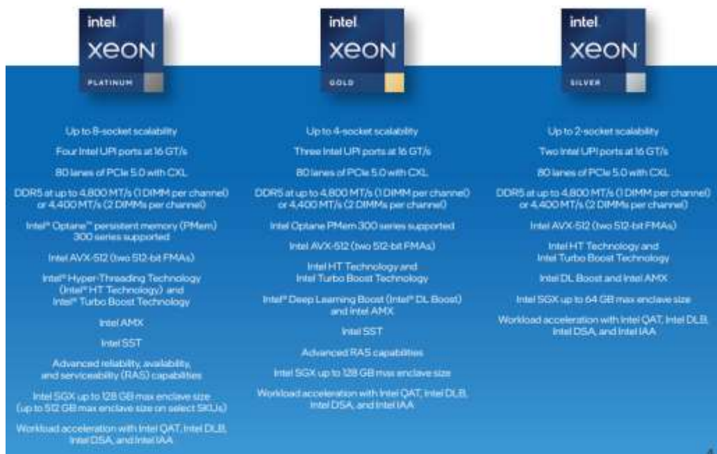
Figure 4.2 Intel Xeon process overview 3
