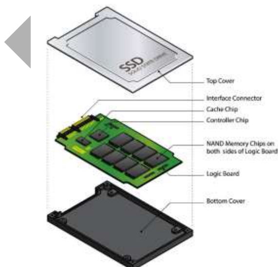
Figure 4.10 Internal components of an SSD 19 .
