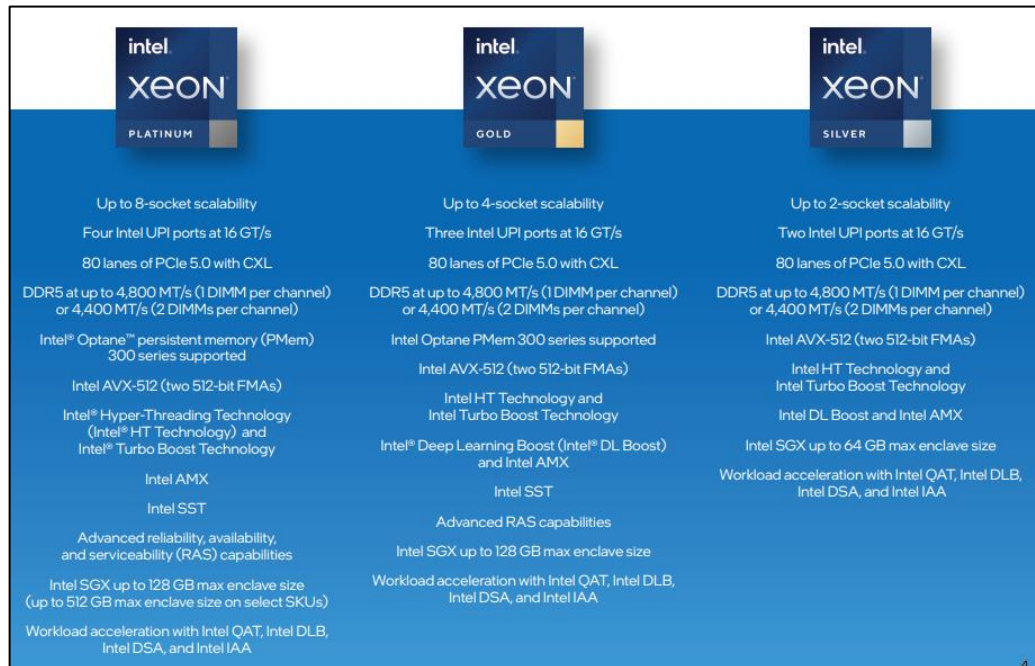
Figure 4.2 Intel Xeon process overview 3
