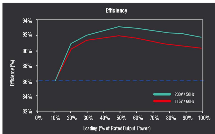
Figure 4.6 An efficiency chart from Cooler Master for their V1300 Platinum PSU
