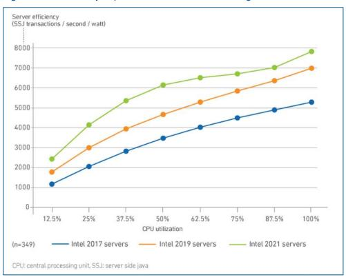
Figure 3.3 Efficiency improves with each Intel server generation<sup>151</sup>
