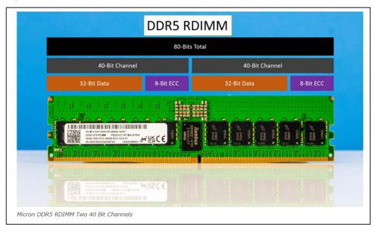
Figure 4.4 Micron DDR5 RDIMM Two 40 Bit Channels<sup>182</sup>
